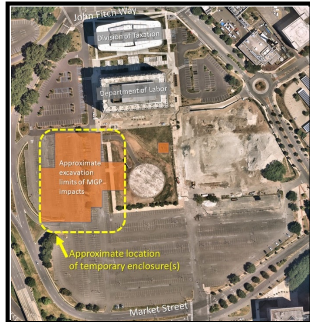
General Area of Future Soil Remediation and Excavation
