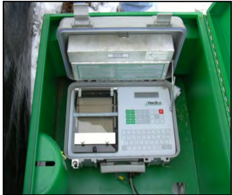
Portable seismograph for vibration monitoring
